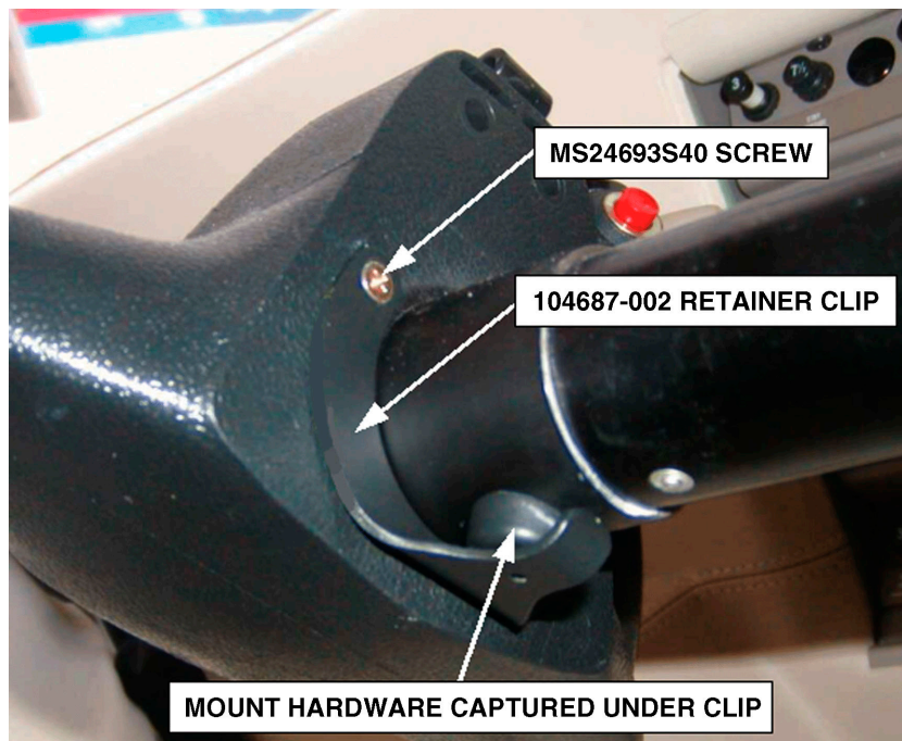
Control Wheel Installation Figure 2
