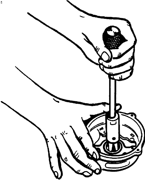
Removing Slip Ring End Bearing Figure 3
